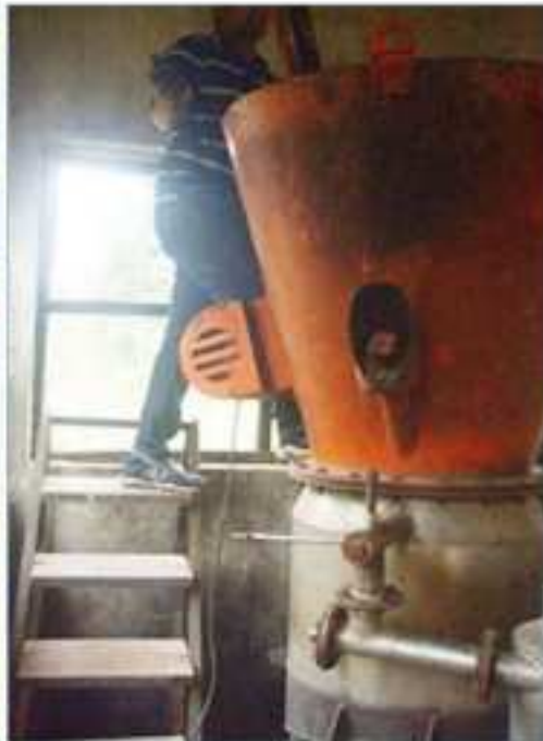
Biomass gasifier for village electrification
